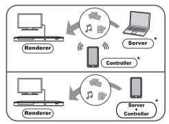
\* DMC compatible software should be installed.
